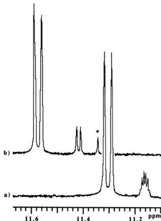
Figure 3. ^1\text{H} NMR spectra of syn and anti alkylidenes of (a) 3b formed upon breakup of metallacycle 2b and (b) 6b formed upon breakup of metallacycle 5b . * = unreacted [\text{Mo}](\text{CHCMe}_2\text{Ph}) .
